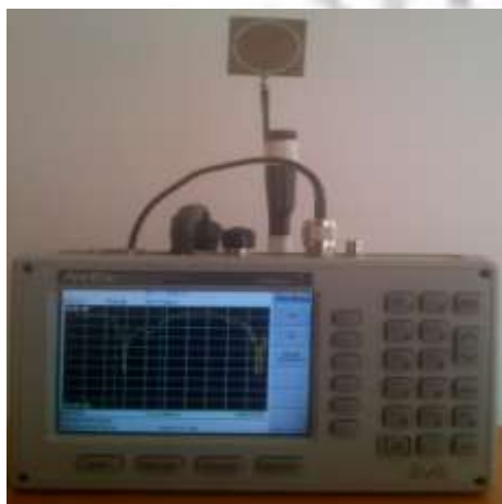
Figure 6 (a): Antenna connected to (Anritsue S332D)
