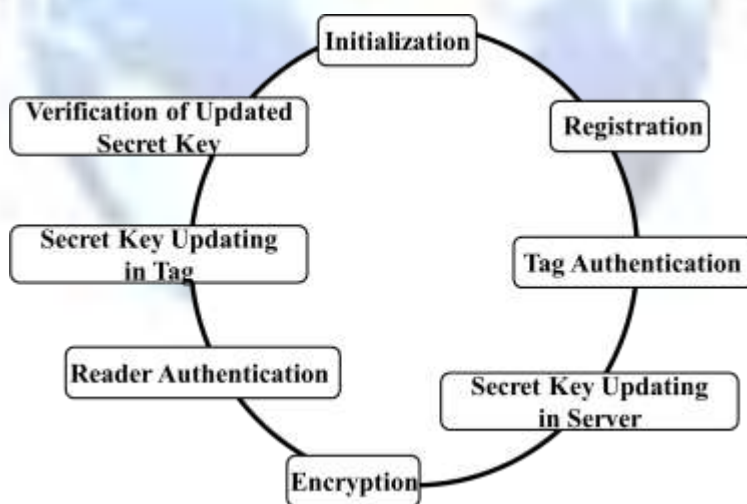
Figure 2. Mobile RFID System Authentication Phase
