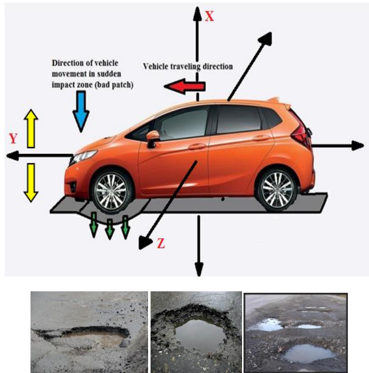
Fig 3: Downward Jerk sensed by Accelerometer which occurred due to above shown potholes over the road
