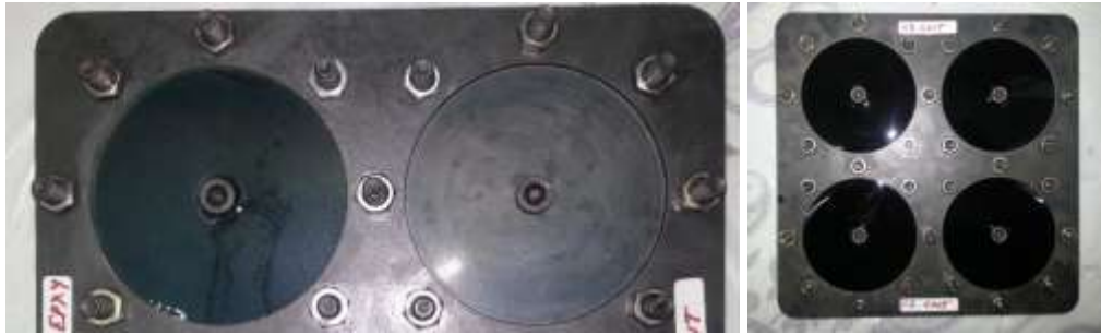
Fig 1. MWCNT composites produced in a steel template
