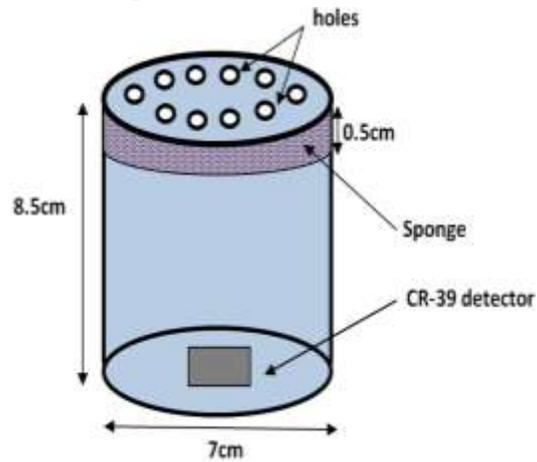
Fig. 1: Schematic diagram showing the geometry of radon dosimeter used in the study (reverse)
