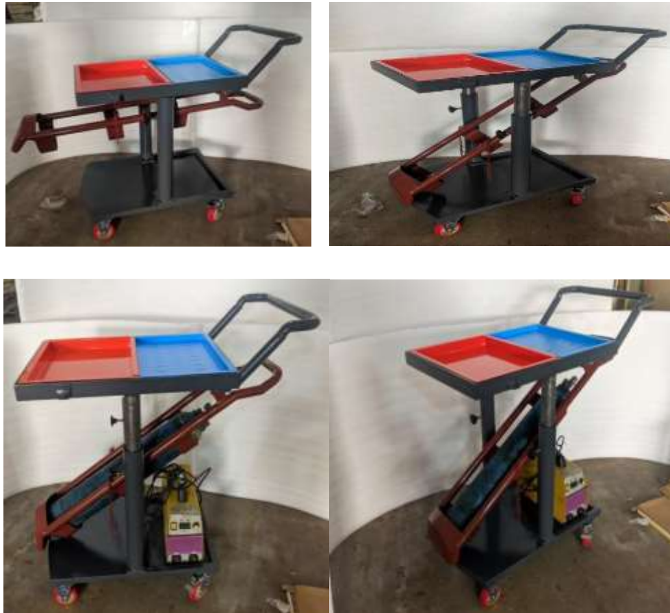
Figure 14 Powder Coated Physical Model with Cylinder and Welding Machine
