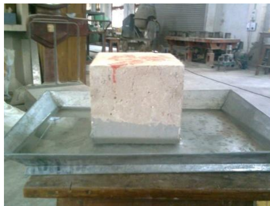
Fig. 4.21 Capillary absorption test of cubes
