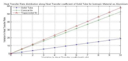
In the above figure Matlab graph is shown which shows the comparative study of Heat transfer rate distribution along heat transfer coefficient between solid tube without fin and solid tube with conical fins & Trapezoidal fins for isotropic material as aluminum.
