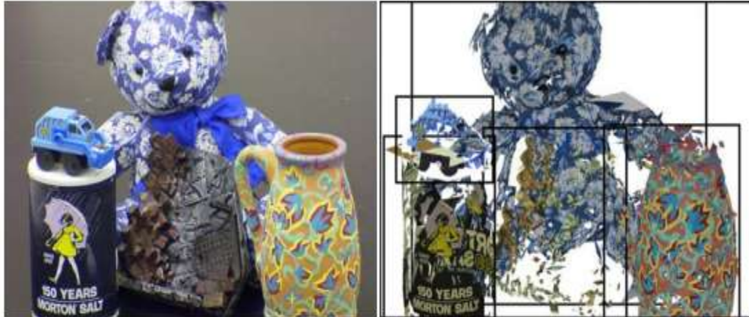
Figure 1. Results of a recognition experiment. Left: A test image. Right: Instances of five models (a teddy bear, a doll stand, a salt can, a toy truck and a vase) have been recognized, and the models are rendered in the poses estimated by our program. Bounding boxes for the reprojections are shown as black rectangles.
