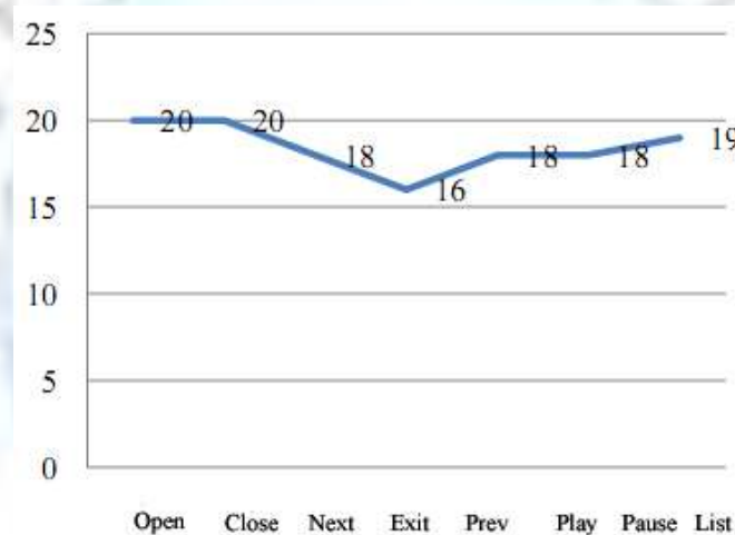
Figure 6: Accuracy Graph of speech recognition circuit
