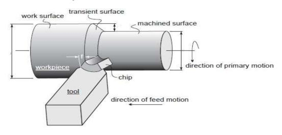
Fig.1- Symmetric view of basic turning operation [IITB]
