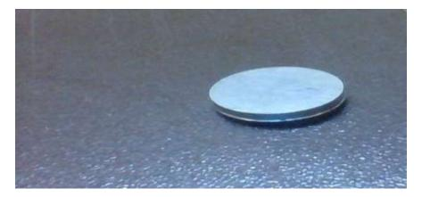
Fig.2-Work-piece specimen material case hardening steel 16MnCr5
