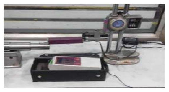
Fig.4-Surface roughness measurement device Mitoyoyo Surf test SJ-201
