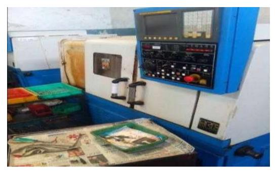
Fig.3- Jobber Junior S designer CNC Turning Centre Machine set up
