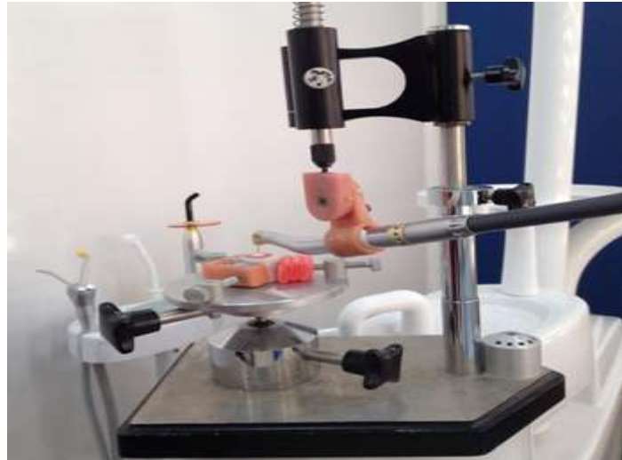
Figure (3): distance between the tip of the laser handpiece and the surface of the zirconium cylinder was 1 mm.
