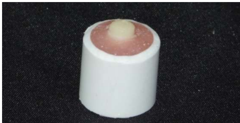
Figure (4): samples after bonding of adhesive cements into zirconia cylinders, the plastic tube was removed
