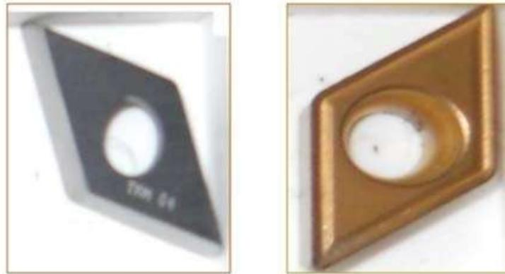
**Fig.2.Uncoated and multilayer coated carbide inserts**
