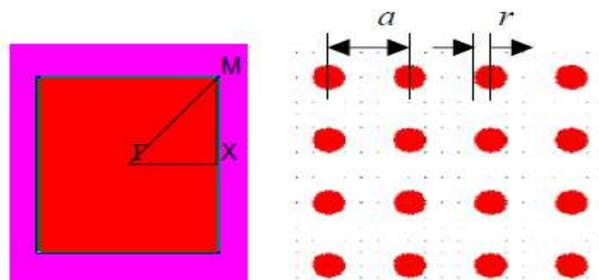
Figure 1. A two dimensional square lattice photonic crystal composed of cylindrical Indium phosphide rods in air, where  $r$  is the radius and  $a$  is the lattice constant of the Indium phosphide rods, respectively.
