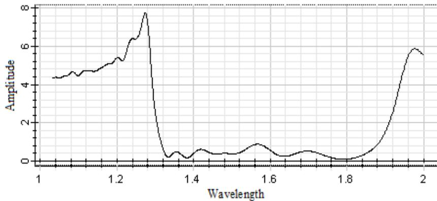
Figure 6. The transmission spectrum of NOT logic gate.
