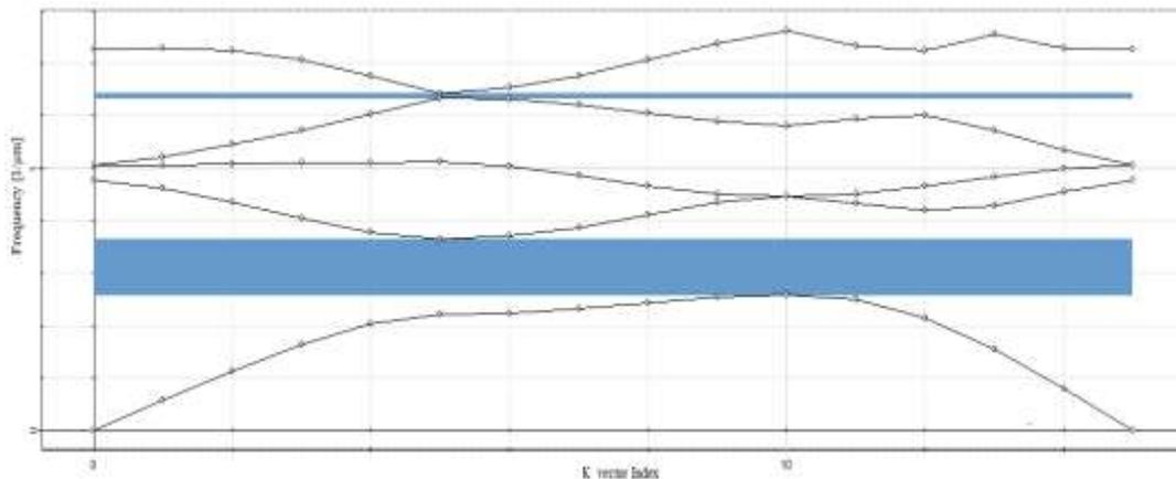
Figure 2. Band gap for NOT logic gate without defect for TE mode
