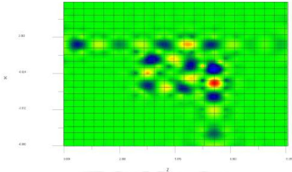
Figure 5 a. The electric field propagation for NOT logic gate when input is 'ON'.
