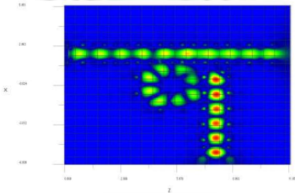
Figure 5.b. DFT of NOT logic gate when input is 'ON'.
