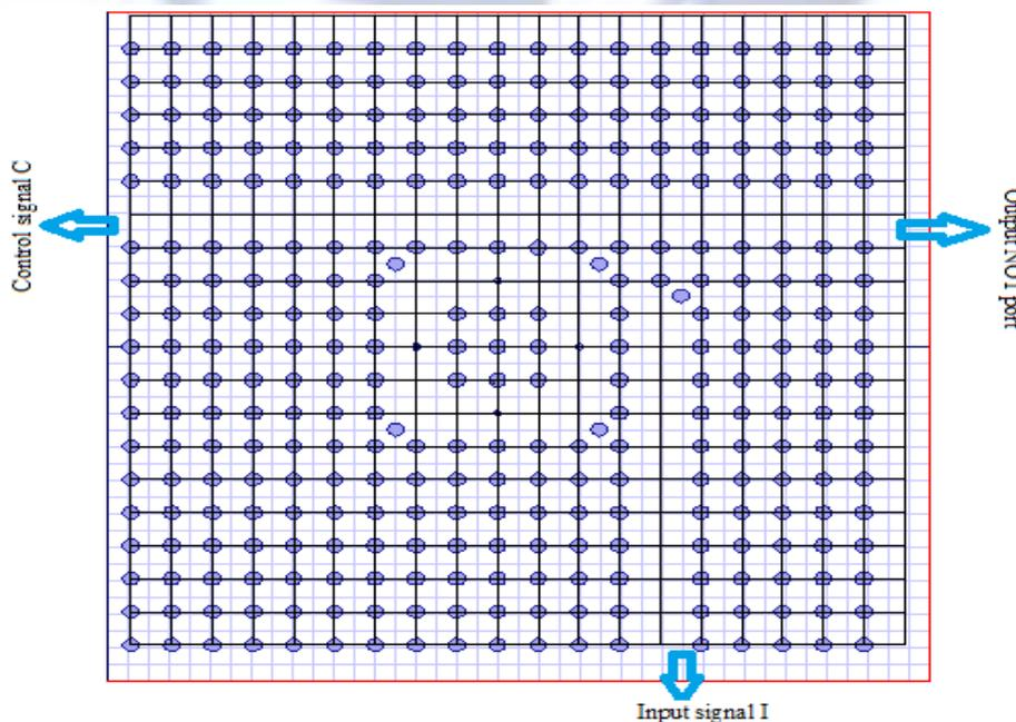
Figure 3 Photonic crystal NOT logic gate structure.
