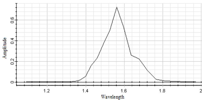
Figure 5 c. Normalised transmission for single wavelength of NOT logic gate when input is 'OFF'.
