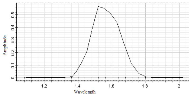
Figure 4.c. Normalised transmission for single wavelength of NOT logic gate when input is 'OFF'.
