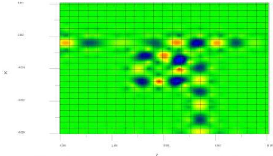
Figure 4.a The electric field propagation for NOT logic gate when input is 'OFF'.
