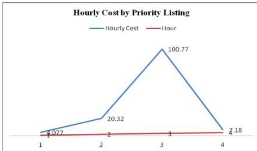
Fig. 3: Graph representing hourly cost in ( \times 10^6 Rs) for 4 hours demand by Priority Listing
