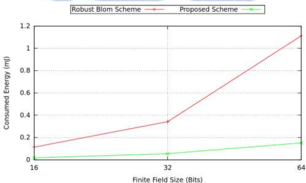
Fig. 3. : Comparison of the amount of consumed energy (mJ) to compute a pairwise key for different key size
