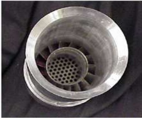
Figure 1 - LSI c/w turbulence grid and swirl blades Image from: [17]
