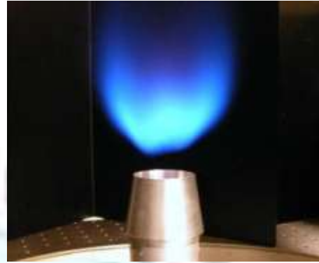
Figure 2 - Detached low swirl flame Image from: [22]
