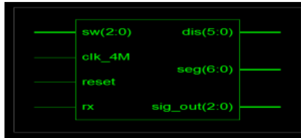
Figure 2.11: RTL Schematic of the Keyboard Interfaced to FPGA Board
