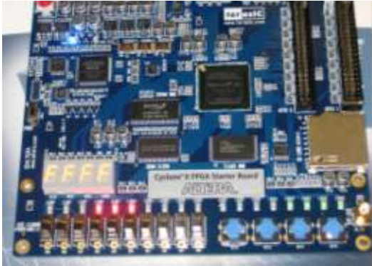
Fig. 3: Device under Test (DUT) - BGA Electronic Package.
