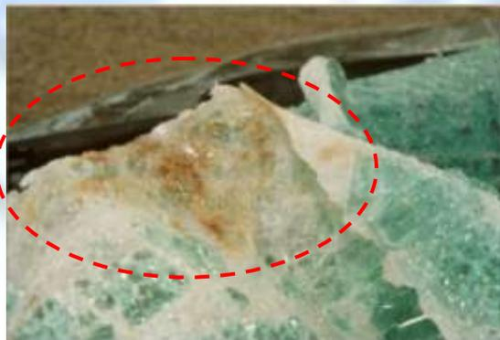
Figure 12. Impact area of windshield with human head produce crack during collision.
