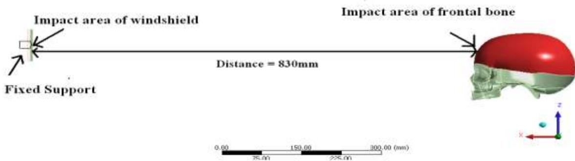
Figure 6. Loading and boundary conditions of frontal skull impact
