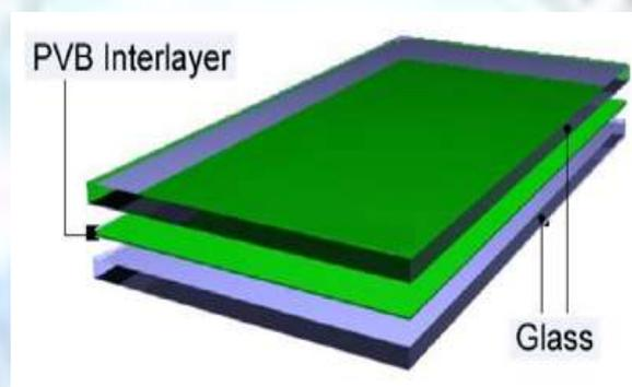
Figure 4. Construction of triple layer of windshield [14].
