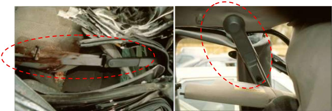
Figure 11. Views of three point belt being locked in a retracted position
