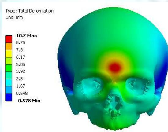
Figure 9. Front view for total deformation of impacted human skull
