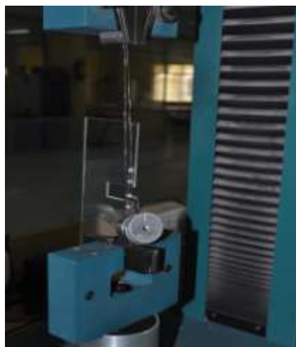
Fig: 1- Jig's placement in UTM
