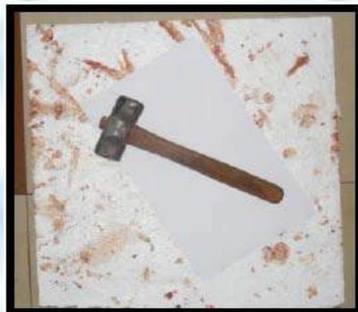
Figure 2: Thermocol sheet placed on the floor to avoid damage of the floor tiles. Paper sheet is placed on the thermocol sheet and hammer is dropped on the paper sheet by measuring the fall height from the top of the thermocol sheet.
