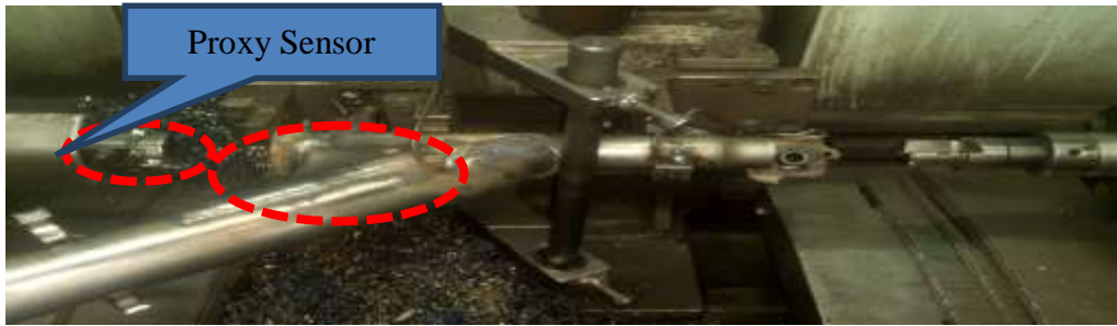
Figure 5 Fine boring Proxy sensor mount on fine boring machine.
