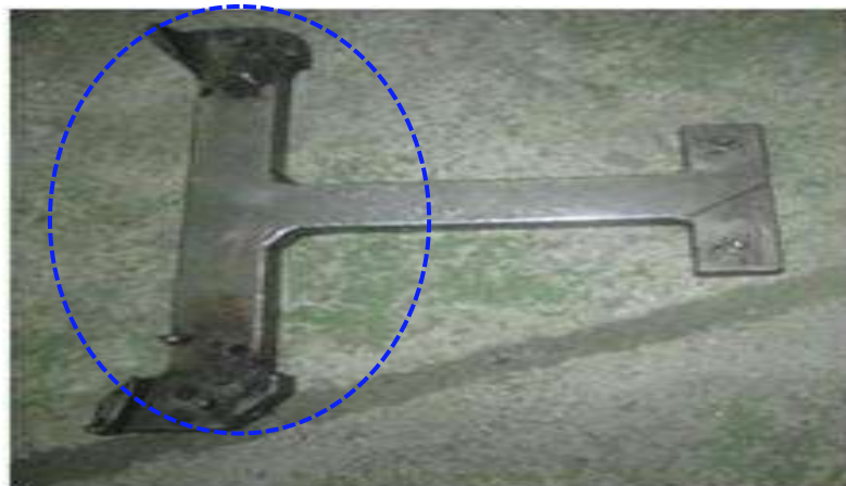
Figure 17 Shown hand jig for holding fuel tank.
