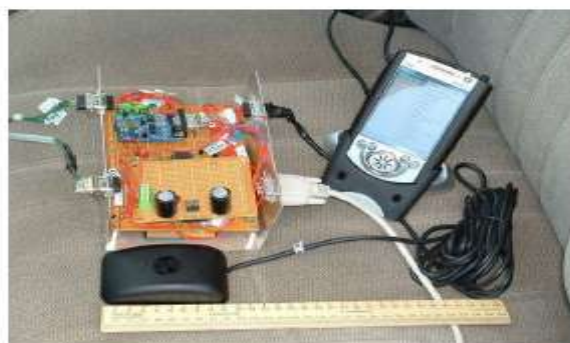
Figure 5. VEDAS system connected to a car. The scantool is connected to the car through the OBD-II connector. A GPS device is connected for location information and the iPAQ downloads the data from the car for analysis [2, Figure 2].
