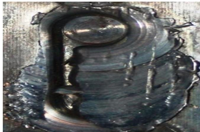
**Fig. 8: Plate melted down at low traverse speed.**
