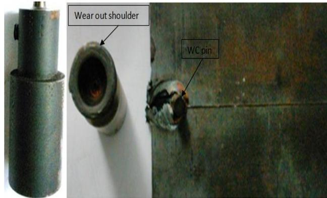
**Fig. 7: Trial tool of tool steel with WC probe and wear out tool.**
