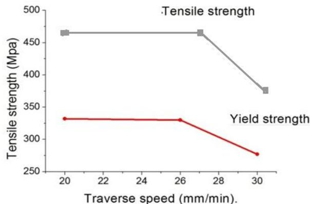
**Fig. 13: Effect of traverse speed on tensile strength.**
