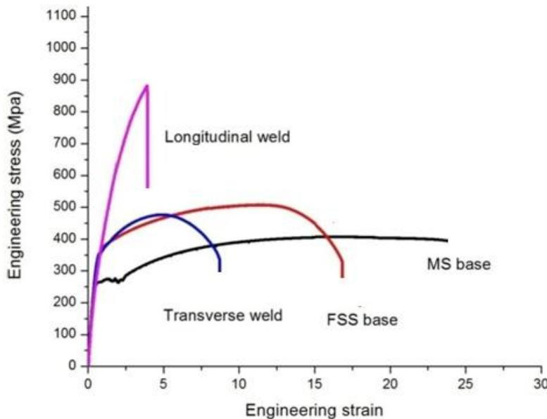
**Fig. 17: Stress Vs Strain curve for FSS welds.**
