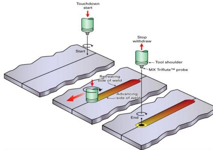
Figure 1: Schematic of FSW [1].
