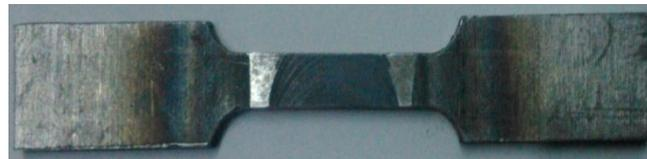
**Fig. 10: Tensile test specimen.**
