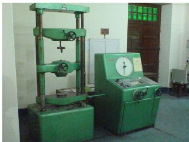
**Fig. 11: UTM used for tensile strength test.**
