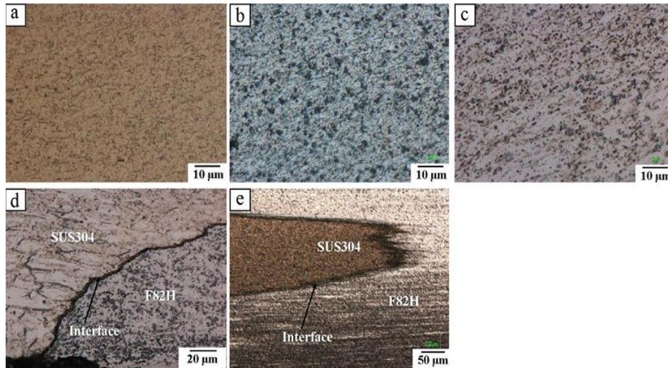
**Figure 3: Microstructures of FSW joint under condition of : (a) stir zone in SUS304, (b) stir zone in F82H, (c) HAZ on the advancing side (F82H), (d) interface in SUS304/F82H and (e) microstructure of SUS304/F82H [11].**
