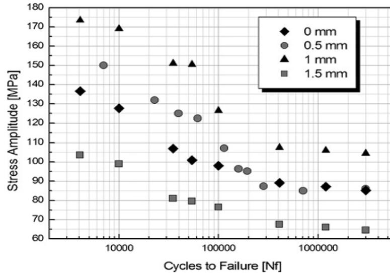
Fig. 5: S–N curves of the different studied joints [23].
