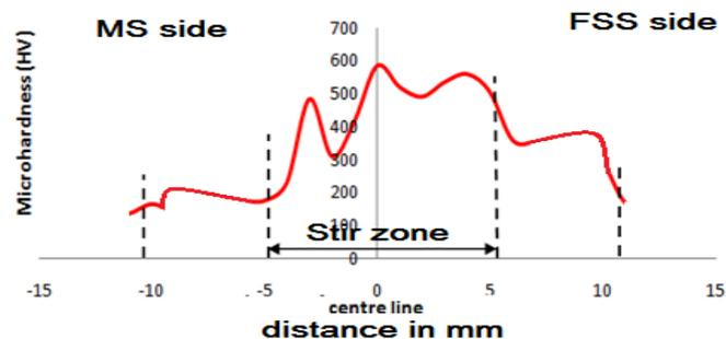
Fig. 15: Hardness profile at the mid thickness of weld.
