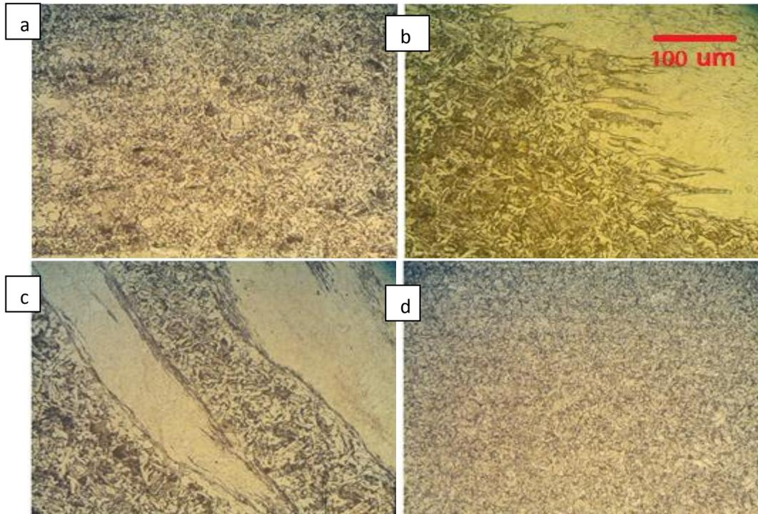
Fig. 14: Optical micrographs of friction stir dissimilar weld a) HAZ of MS, b) metal flow in stir zone, c) interface between MS and FSS and d) HAZ of FSS side.
