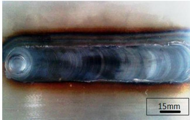
**Fig. 12: Weld appearance without surface defect.**
