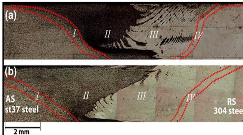
Figure 2: Different micro structural regions in the cross-section of the welds [10].
