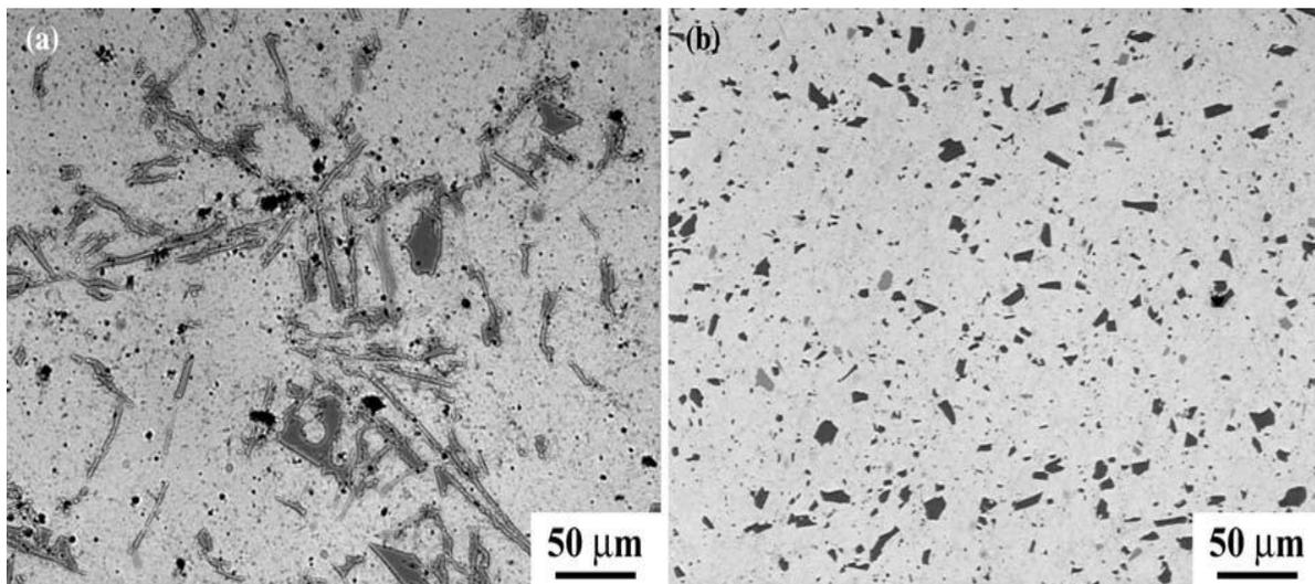
**Fig. 4: Optical micrographs showing morphology and distribution of Si particles in A356 samples: (a) as-cast and (b) FSP at 900 rpm and 203 mm/min.[3]**
