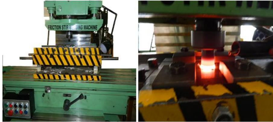
**Fig. 9: FSW machine during the weld.**
