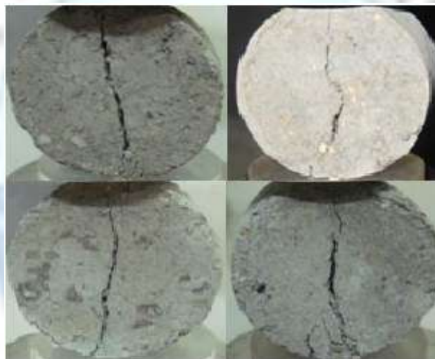
Figure 5 : Post failure profiles of a few tensile test specimens
