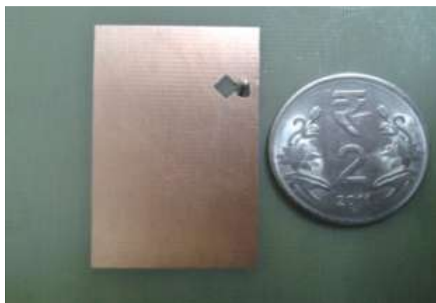
Fig. 4: Fabricated Rectangular Patch Microstrip Antenna with Shifted Rhombus Slot (RPMASRS)
