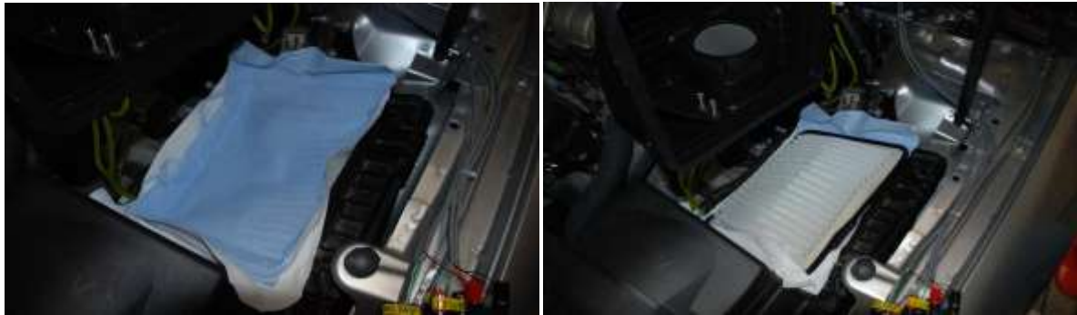
Fig. 2.5: filter restriction. Shop towels inserted into air box upstream of the air filter.
