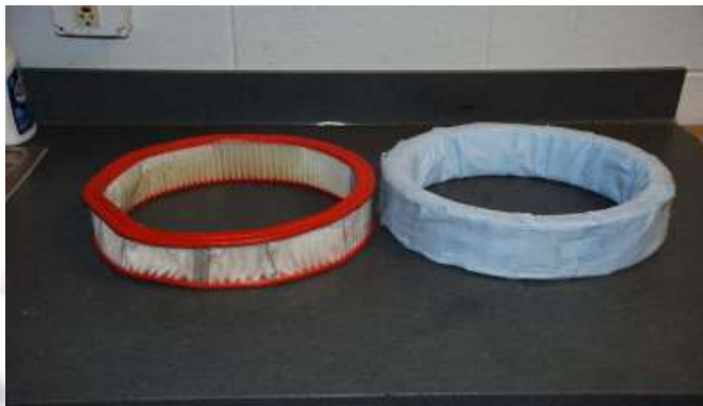
Fig. 2.6: 1984Super Saloon air filter. Filter on the left shows damage that occurred during “severely clogged” filter testing
