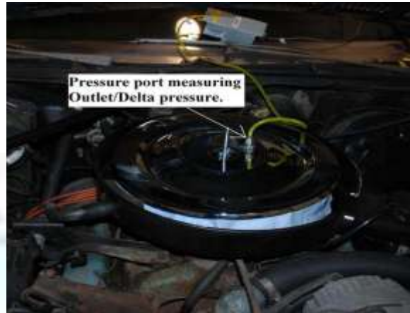
Fig. 3.9: Pressure port location for 1984 Super Saloon
