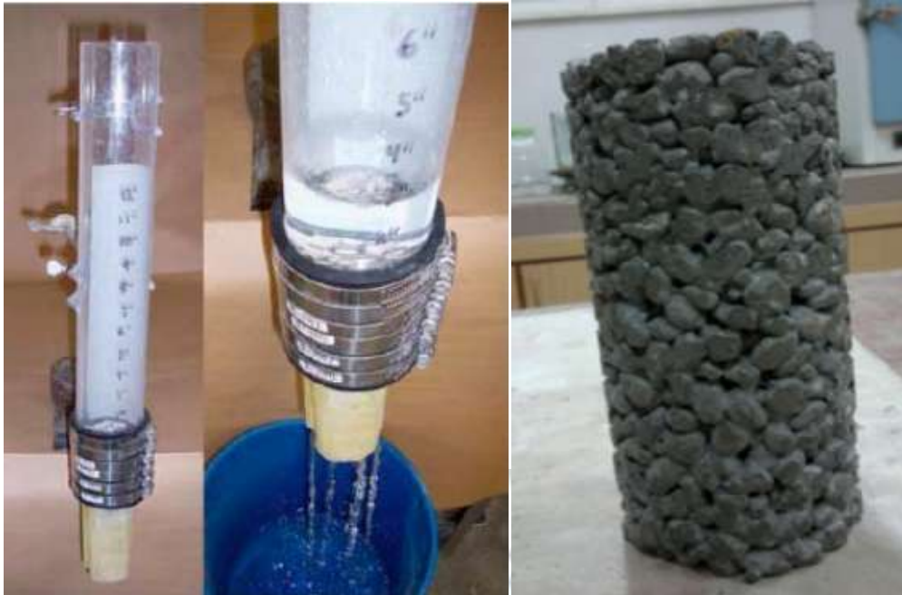
Figure 1. Falling Head Permeability Test for Pervious Concrete.
