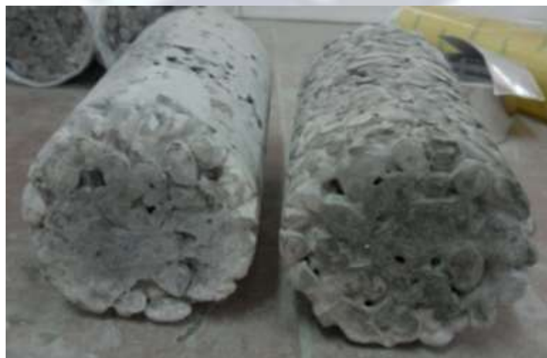
Figure 3. (Mix.4) Clogging Bottom of Sample Pervious Concrete because of use High too much Water
