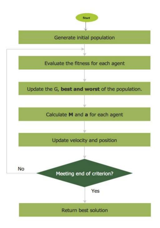
Fig.2: Flow Chart of Gravitational Search Algorithm for Wind-Thermal Scheduling
