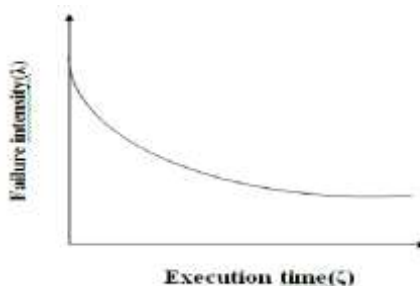
Fig 5: Failure intensity versus execution time for basic model
