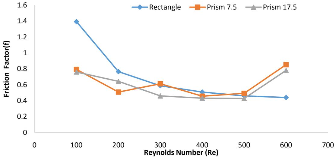
**Fig 3.8: Friction factor Vs Reynolds number**
