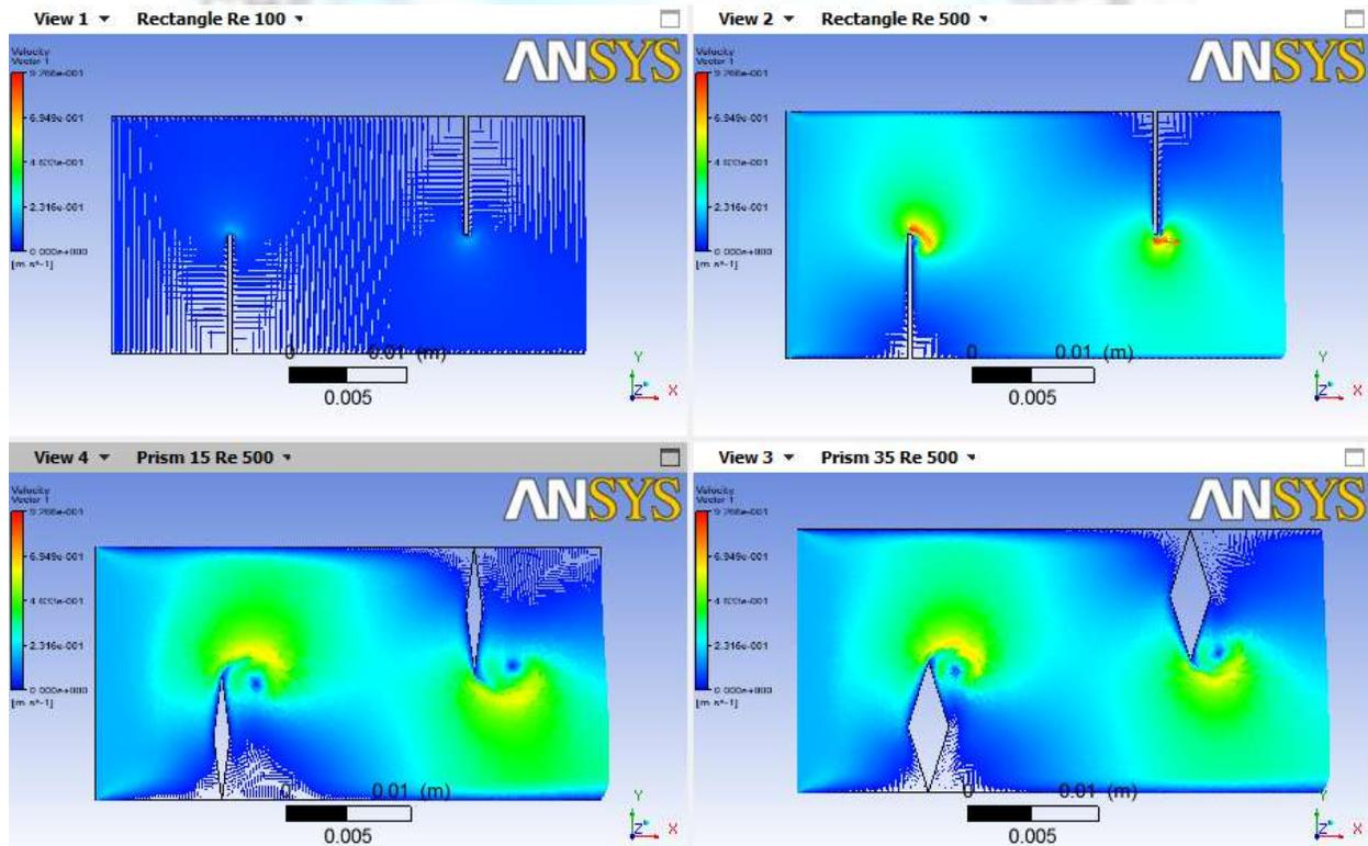
Fig; 3.1 Velocity vector for Prism baffle ( $2\theta=15^\circ, 35^\circ$ ) and rectangle baffle
