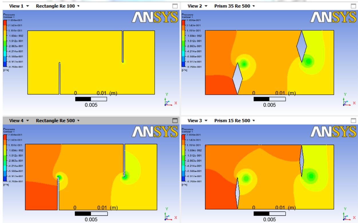
Fig; 3.3 Pressure contour for Prism baffle ( $2\theta=15^{\circ}, 35^{\circ}$ ) and rectangle baffle
