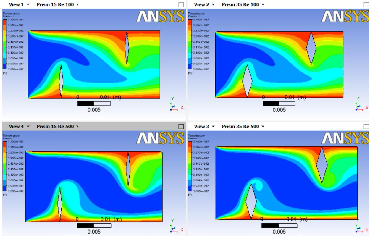
Fig; 3.2 Temperature contour for Prism baffle ( $2\theta=15^{\circ}, 35^{\circ}$ ) at Reynolds no. 100 & 500
