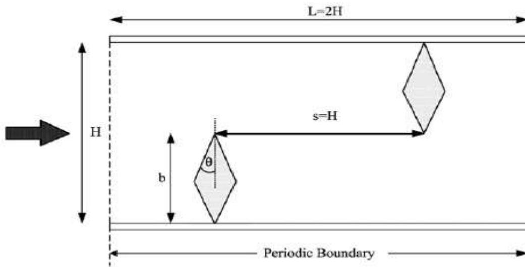
Fig 2.1 Channel geometry and computational domain of periodic flow.
