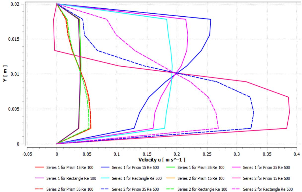
Fig. 3.4: Axial velocity profiles at  $x=0.02$ (Series=1) and  $x=0.035$ (Series=2) for  $re= 100 \& 500$
