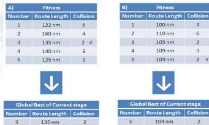
Figure 13. Step-by-step selection of local best for each member using old local best and fitness in present stage.
