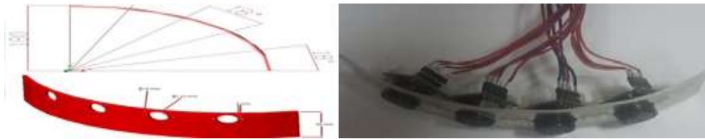
Figure 3. Sensors Arc mounted on Gondola
