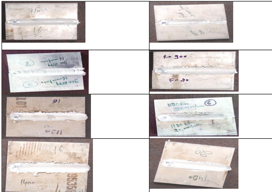
Fig. 3 Friction stir welded AA6061-T6 alloy specimens
