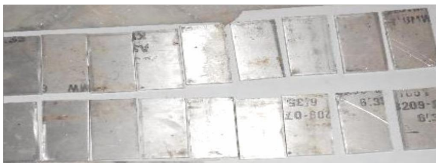
Fig. 2 Test specimens of aluminium alloy AA6061-T6
