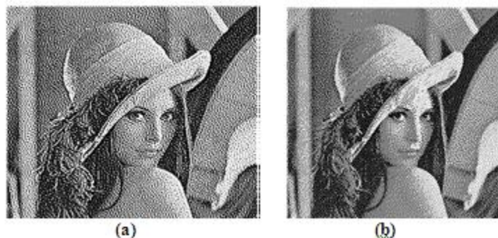
Figure 13: Halftoning image by Error Diffusion. (a) Using weight matrix 12(a). (b) Using weight matrix 12(b)
