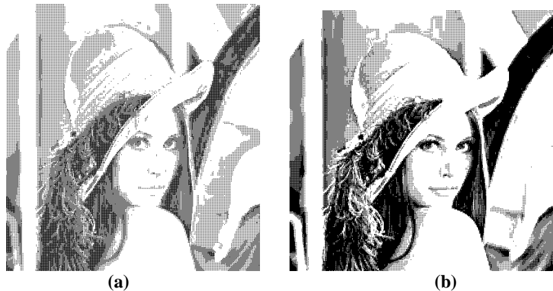
Figure 10: Halftone images by block replacement. (a) The candidates are 2 x 2, i.e. 5 gray levels (b) The candidates are 3 x 3, i.e. 10 gray levels.
